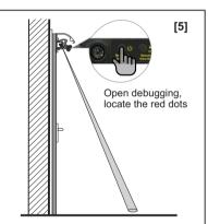
Open the debugging positioning red dots, confirm the general position of the sensing beam(Red dots isn't laser beam, laser beam is invisible light)
