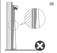
When install it on the door leaf, recommended that the tilt angle of sensor will be ≥15°, ensure laser beam doesn't scan the door leaf, sensor detection will be more stable.
