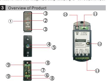
① LED indication (red light flashes in the power-on learning state, the red light flashes when standby, and the action blue light is on)
