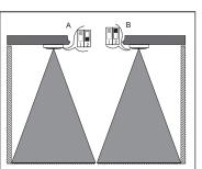
When two sensors installed in very close position, Sensors should be set to different rates. One senso with A ,Antoher one with B.(as picture)
