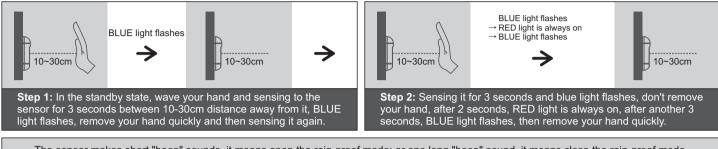
The sensor makes short "beep" sounds, it means open the rain-proof mode; or one long "beep" sound, it means close the rain-proof mode.
