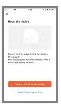
Step 5: Press and hold the sensor's function button until the Blue indicator light flashes, after 10 seconds and Green indicator light will quick flashes, then click "Confirm the indicator is blinking rapidly" on the phone interface.
