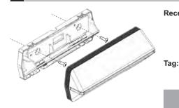
Receiver: 1. Pry and open the housing by a screwdriver along the notch on the bottom of the receiver.
