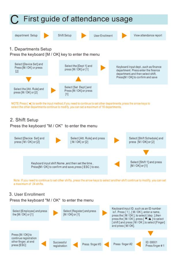
Note: The same ID number can register up to 10 fingerprints. You can also choose Password, Card, Face or Palmprints registration, and the password length is set to 8 digits. Face and palmprint need to be recorded 8 times in turn.
