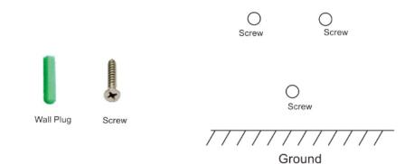
2.Hang the machine on the hanging board on the wall and tighten the bottom hanging board screw to complete the installation
