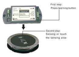
Attention: Since the system has learned the current sensing touch environment when the battery is installed, when fixing it to the wall, it may appear to be in the sensing status. Don't sensing or touch the panel at this time, after 16 seconds the system will re-learn the touch environment.
