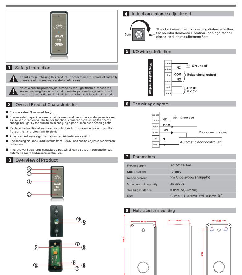
① LED indicator (standby red light flashes for 1.5 seconds, action blue light flashes)
