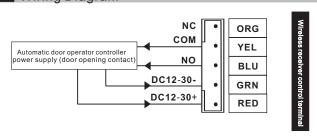
Wiring diagram of wireless receiver control automatic door operator
