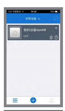
Step 14: You will see the equipment on this page. Press it to output DOOR OPEN signal.
