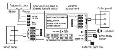
The inner and outer panel wiring are the same.
