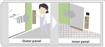
[ 2 ] wave hands to the door open button on the outer panel, and the automatic door open. At the same time, there is a voice prompt "door is opening".
