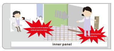
[7] The longest use time of this system is 30 minutes. When using it for 25 minutes, the system will voice prompt "This system will unlock the anti-lock function in five minutes. If you need to continue to use, please press the confirmation button, thank you" otherwise the system will be in five minutes Automatic unlocking
