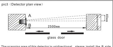
The scanning area of this detector is unidirectional, please install the B side close to moving things to avoid self-inductance.
