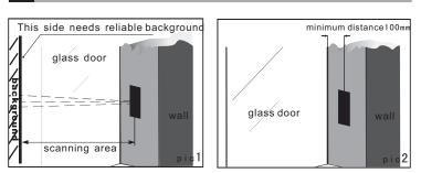
note: The background towards detector note: The minimum distance between must be reliable and stable. Or it will lose door and detector is 100mm. scanning signal.
