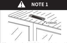
When top suction installation, in order to avoid self-induction, the installation distance between the automatic door and the safety cutain should be more than 100mm.
