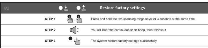
Restore data includes: 1, Scanning range return to the 4th level; 2, Working mode returns to normal mode; 3, Test signal output is high output active; 4,Output signal is NC signal.
