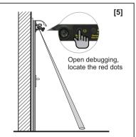
Open the debugging positioning red dots, confirm the general position of the sensing beam(Red dots isn't laser beam, laser beam is invisible light)
