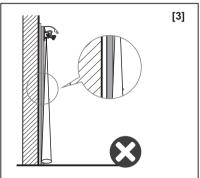
When install it on the door leaf, recommended that the tilt angle of sensor will be ≥15°, ensure laser beam doesn't scan the door leaf, sensor detection will be more stable.
