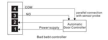
Wiring diagram of connecting with autodoor
