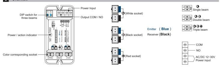
**NOTE:** Open the front cover, find the dip switch, transmitting electric eye(blue cable) and receiving electric eye(black cable). For single beam, it must connect to A group of white socket, double beams, it must connect to AB group of white and black socket, triple beams, it must connect to ABC group of white and black and red socket.
