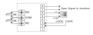
Lock signal of access to unlock the electric bolt and open door
