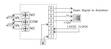
Exit switch to unlock the electric lock and open door
