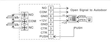
PUSH Signal to unlock electric lock and open door
