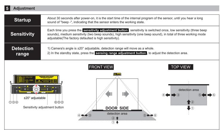
3) Every time you press the sensing range adjustment button, the detection range of the every corresponding edge (as shown in the figure) will move 1 level, total of 10 levels, until the sensor have beep beep sounds, means the detection range has been adjusted to limit, the limiting position of edge ③⑤ is center line.
