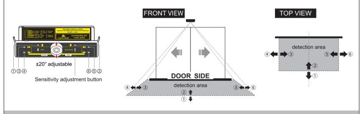
3) Every time you press the sensing range adjustment button, the detection range of the every corresponding edge (as shown in the figure) will move 1 level, total of 10 levels, until the sensor have beep beep sounds, means the detection range has been adjusted to limit, the limiting position of edge ③⑤ is center line.
