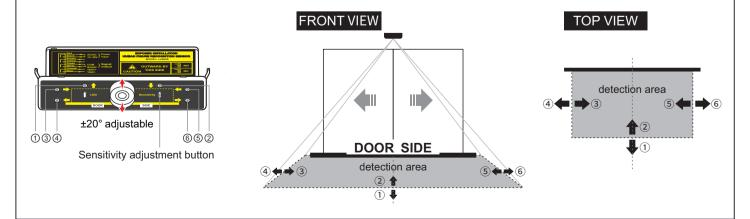
3) Every time you press the sensing range adjustment button, the detection range of the every corresponding edge (as shown in the figure) will move 1 level, total of 10 levels, until the sensor have beep beep sounds, means the detection range has been adjusted to limit, the limiting position of edge ③⑤ is center line.
